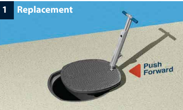
Push back the cover into the frame with the aid of the lifting tool and your foot if necessary. Step down on the cover to re engage the seal.
