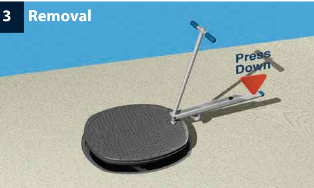
Release the seal breaker from the lifting tool and press down on the foot pedal to release the cover from its frame.
