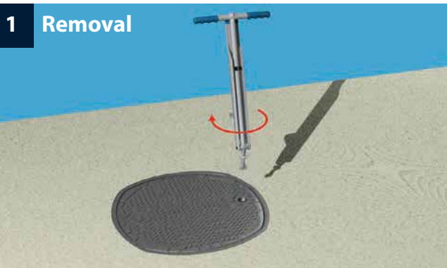
Insert the lifting tool into the lock aperture as shown above and turn the handle through 90° clockwise towards you.
